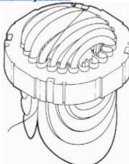
This is still the most economical process for the quick, quality insertion of the coil groups into the stator slots. It uses highly polished tool steel to cover the saw tooth edged stator slot opening from the incoming wires. As the wire is pushed into the slots, the slot closure wedge follows the wire up through the tooling (additional information is available at http://www.alliance-winding.com).
